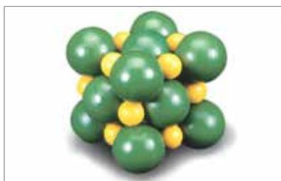
Fig. 5: Cristal NaCl
