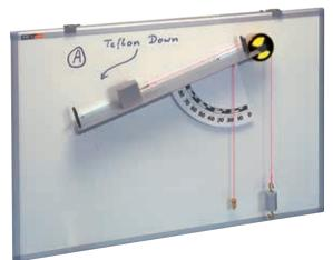
Friction on an inclined plane
