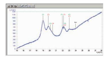
Collector current  $I_{\rm R}$  as a function of accelerating voltage  $U_{\rm A}$ . Gas filling: He.
