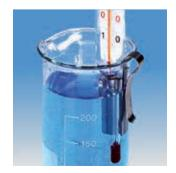
Thermometer Clip Stainless steel clip for holding thermometers in beakers. P-1003528
