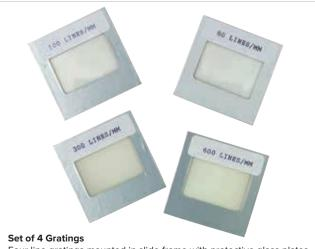
Four line gratings mounted in slide frame with protective glass plates.
