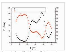
Transmission of light from a diode through an Nd:YAG crystal as a function of temperature for various injection currents
