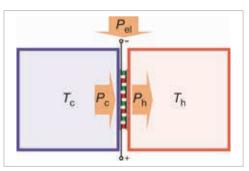
How a Peltier heat pump works
