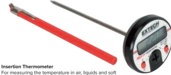
For measuring the temperature in air, liquids and soft materials. Temperature sensor made of stainless steel with protective case, switchable between °C and °F, On/Off switch and automatic switch-off.
