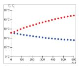
Change of temperature over time in both reservoirs during
