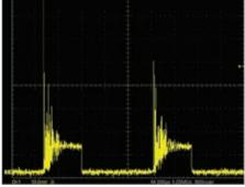
Oscilloscope trace: spiking in a Nd:YAG laser
