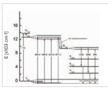
Energy level diagram for an Nd:YAG crystal with the most important transitions for optical pumping and laser operation
