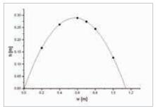
Oblique launch: projectile height as a function of the projectile distance (launch angle: 45°)
