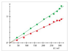
Angle of rotation as a function of the magnetic field for red and green laser light
