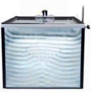
Refraction of water waves at a converging lens
