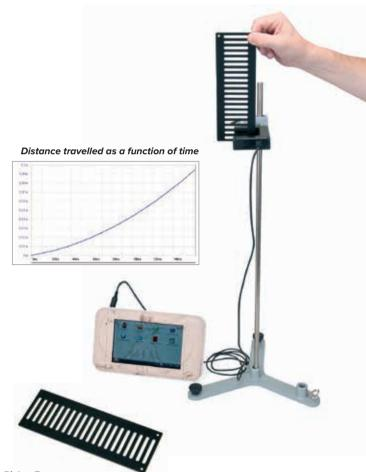
The picket fence is used to determine gravitational acceleration g in conjunction with the light barrier (P-1000563). It consists of anodized aluminium sheets with 21 crosspieces and two boreholes for suspending additional masses.
