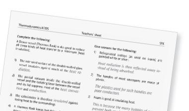
This is because the many bubbles of air prevent both conduction and convection of heat.
