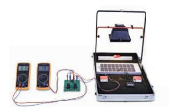
How power output from solar modules depends on temperature
