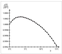
Determining the maximum density of water
