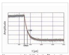
Measurement of half-life for the  ${}^4F_{3/2}$  level in an
