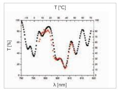
Comparison of transmission functions: Square- T(λ) recorded using a spectrometer Triangular - Transmission as a function of temperature
