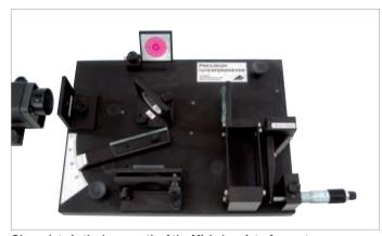
${\it Glass\ plate\ in\ the\ beam\ path\ of\ the\ Michelson\ interferometer}$
