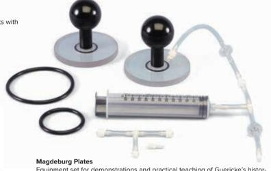
Equipment set for demonstrations and practical teaching of Guericke's historical experiment investigating the effect of atmospheric pressure. Includes nozzle for tubing, a simple hand pump and tubing with built-in directional valves. Two transparent acrylic plates with handles that can be held together with a coarse vacuum between them. Three sealing rings of various sizes are supplied for sealing the plates. This allows the dependency of the force on the contact area to be investigated.
