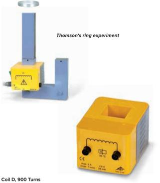
Coil with 900 turns and thermal overload protection. For generating powerful magnetic fields in conjunction with the U-core (P-1000979).
