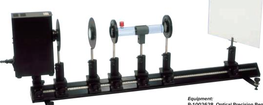
Determination of the angle of rotation of optically active substances
