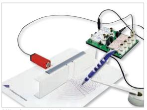
Diffraction by a double slit
