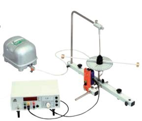
Measuring the period of oscillation and determining the moment of inertia
