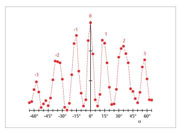
Intensity distribution resulting from the diffraction of microwaves at a pair of slits
