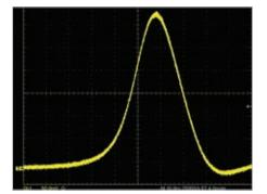
Oscilloscope trace: trace of pulses from a passive Q-switched Nd:YAG laser. Pulse duration 25 ns
