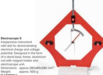
electroscope unit. Dimensions: approx.280x80x280 mm<sup>3</sup> Weight: approx. 500 g P-1009964
