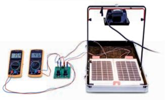
Current-voltage characteristic for solar modules in series
