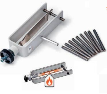
Demonstrate the forces resulting from changes in length arising from heat or cold. These forces are sufficient to break a 10-mm iron bolt.
