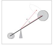
Schematic of a gyroscope illustrating nutation
