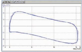
Pressure-volume diagram of Stirling engine D
