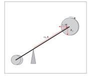
Schematic of a gyroscope illustrating precession
