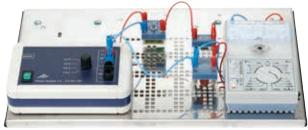
Charging and discharging of a capacitor (voltage)
