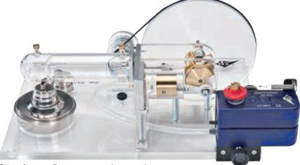
Set-up for recording a pressure-volume graph
