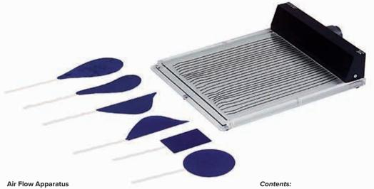
Apparatus for demonstrating air flow patterns around bodies of different shapes. The air flow patterns can be projected on to a wide screen using an overhead projector. Two strings are fastened on one side at equal distances between two glass plates. The strings move according to the air currents between the two glass plates. Bodies of different shapes can be introduced in the air current. The inserted bodies can be moved to various positions in the air current from outside. Includes a hose.
