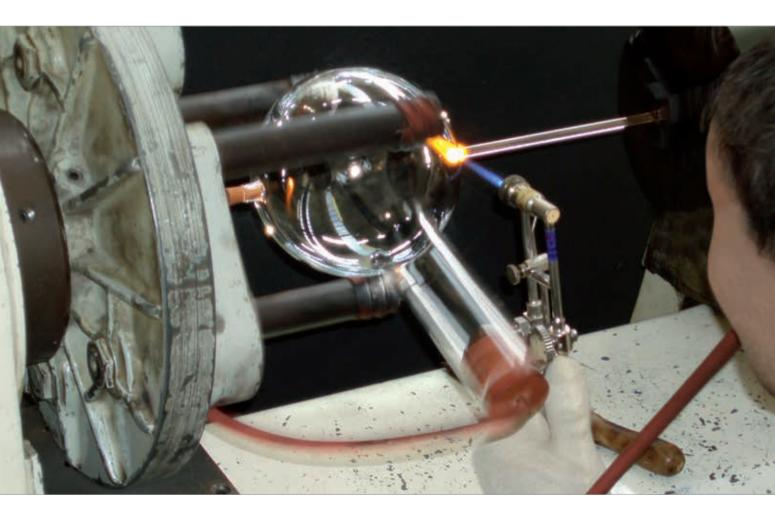
Manufacturing a TELTRON® electron tube at 3B Scientific in Germany Electron tubes are produced at only a very small number of places in the world. Only specially trained technicians with many years of experience have
