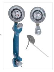
measurement accuracy and repeatability. Includes a 90.7 kg hydraulic hand dynamometer, 22.7 kg hydraulic pinch gauge and stainless steel finger goniometer.
